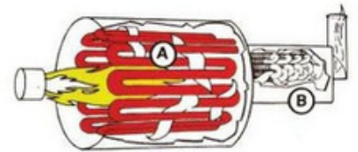
SERPENTINE COIL HEATER WITH CONVECTION SECTION (ECONOMIZER)
